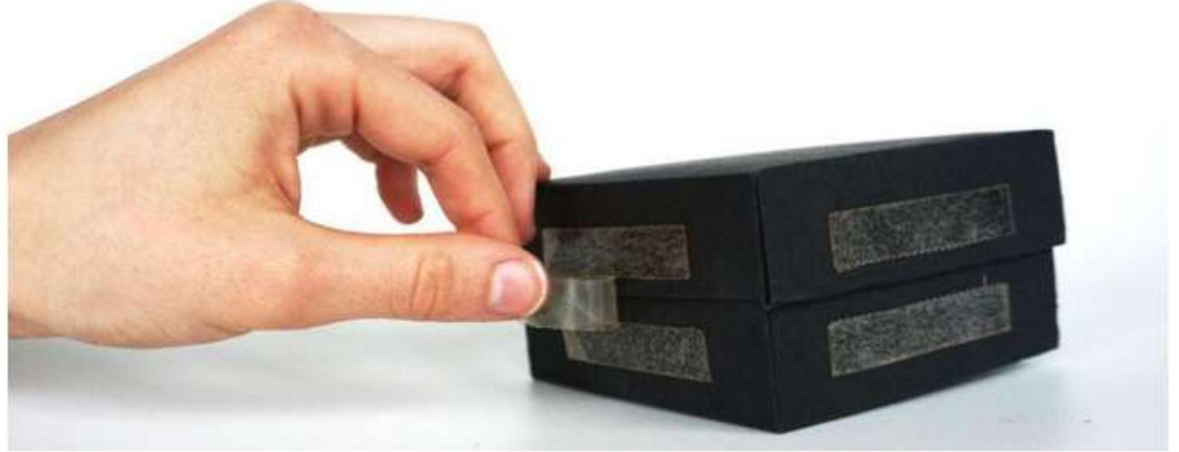
The result is MarinaTex, a bioplastic film made primarily from fish scales and skins and bound with an organic binder. Creating MarinaTex required a lot of trial and error, but the result is more than a polymer; MarinaTex is biodegradable plastic sheeting that is versatile and naturally decomposes in 4 to 6 weeks in a home **compost** environment.
